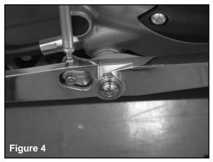
Install the electric shift cylinder onto the electric shift cylinder to engine support bracket using the Pingel clamp and (2)  $\frac{1}{4}$ -20 x  $\frac{3}{4}$ " socket head cap screws, adjusting the cylinder so the clamp is approximately  $\frac{1}{4}$  of the way down from the top (see figure 3). Just snug these bolts for now, as adjustment will be needed.
